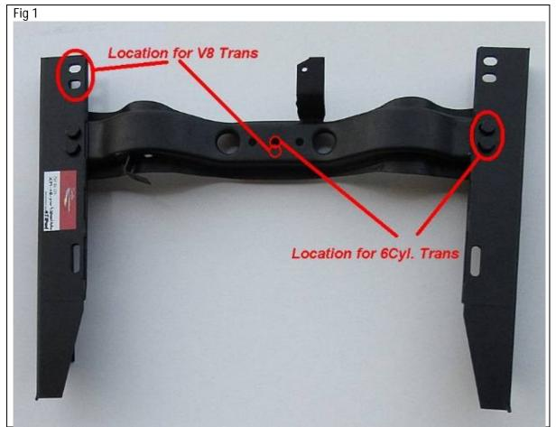
To fit the longer transmissions a hole must be drilled in the centre of the Original rear crossmember as shown in Fig 1.
